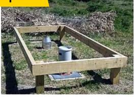
The weather station provides real-time monitoring of rainfall, wind speed and direction, relative humidity, and temperature and barometric pressure. The data can be viewed through the Regional Council's live monitoring website and will also be available on the MetService website soon
