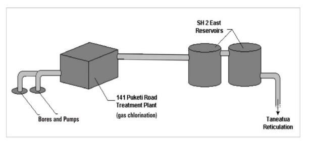
A schematic of the water supply is illustrated below. Note that the clorination plant now also includes UV treatment.
