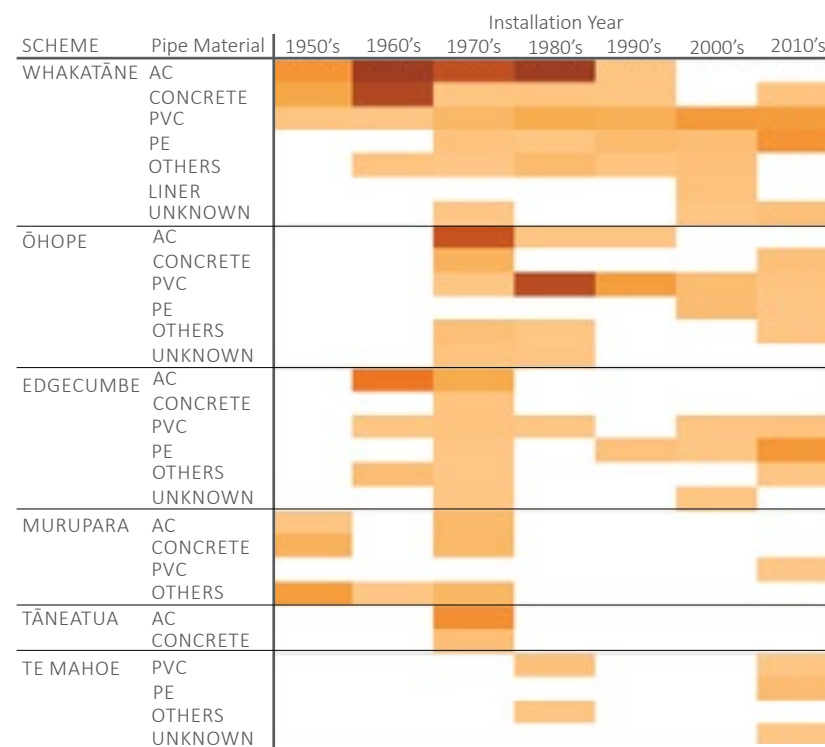
Figure 1: Pipe material and age for each scheme
