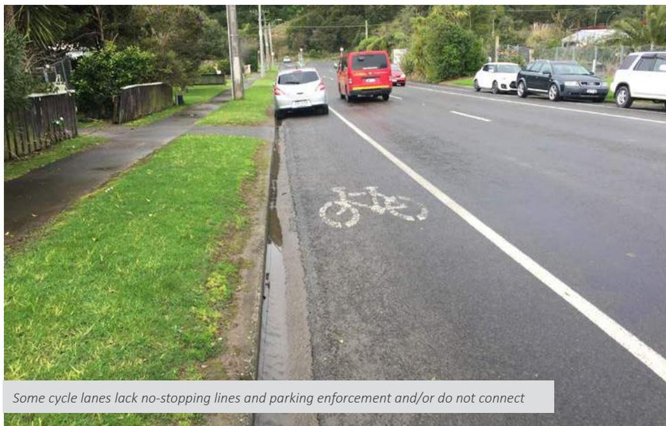
*Some cycle lanes lack no-stopping lines and parking enforcement and/or do not connect*
