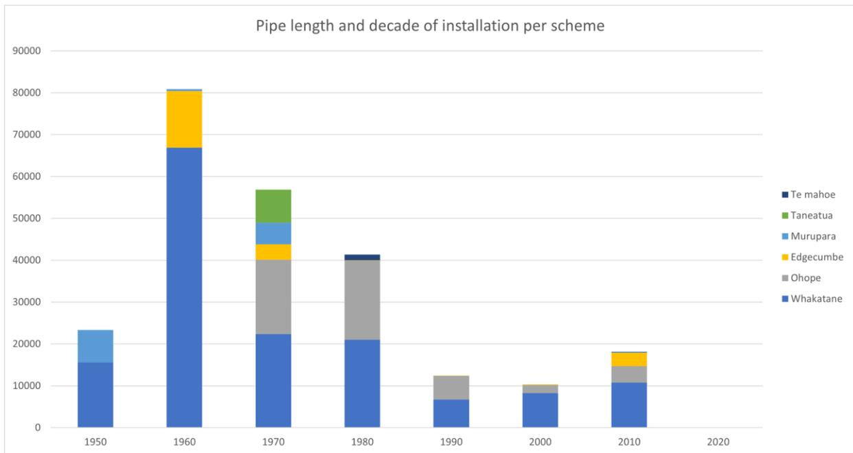
Figure 8 – Age profile of wastewater piped asset.
