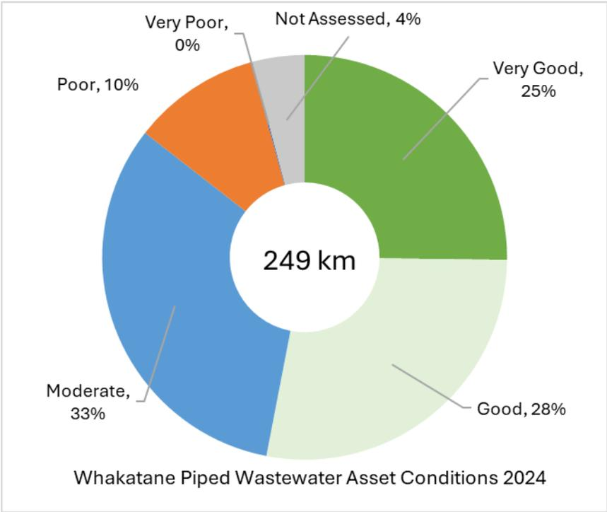
Figure 7 – Wastewater piped assets condition ratings.
