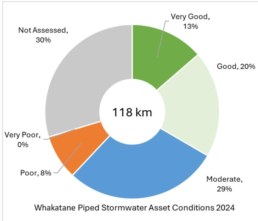
Figure 5 – Stormwater piped assets condition ratings
