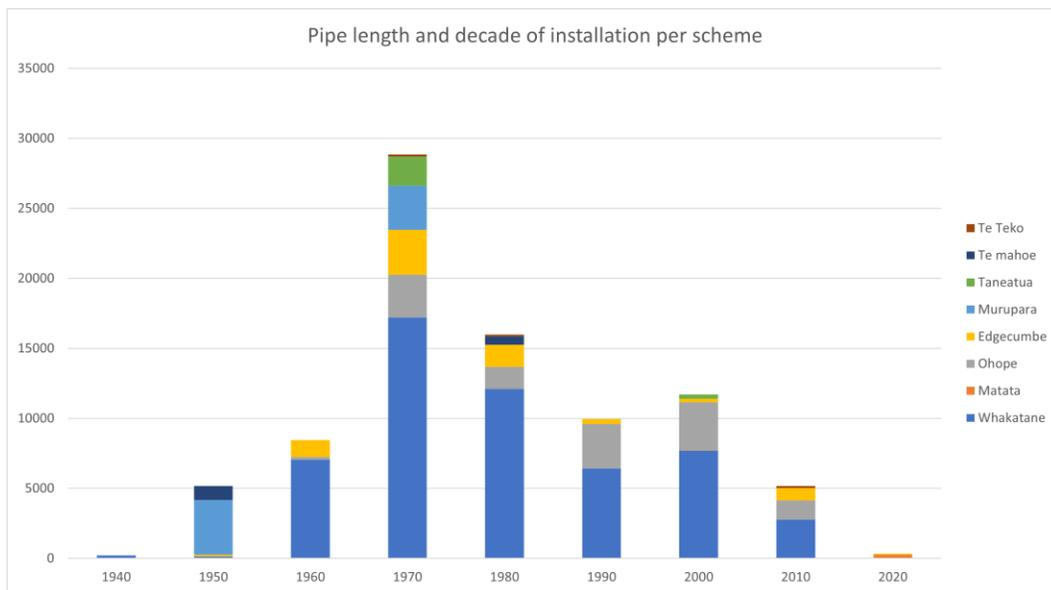
Table 8 – Age profile of piped stormwater asset
