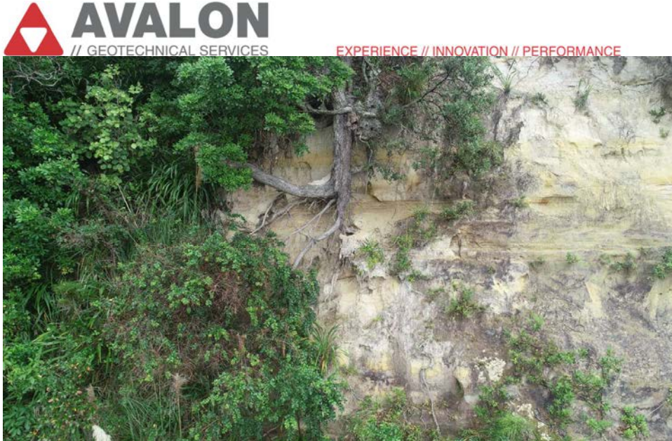
Left of face above track at slip 2 typical conditions large overhanging Pohutukawa root
