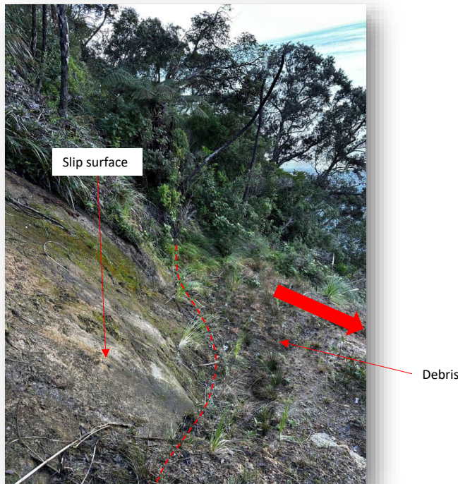
Photo 12: Transition from slip surface to debris that is hung up on slope.
