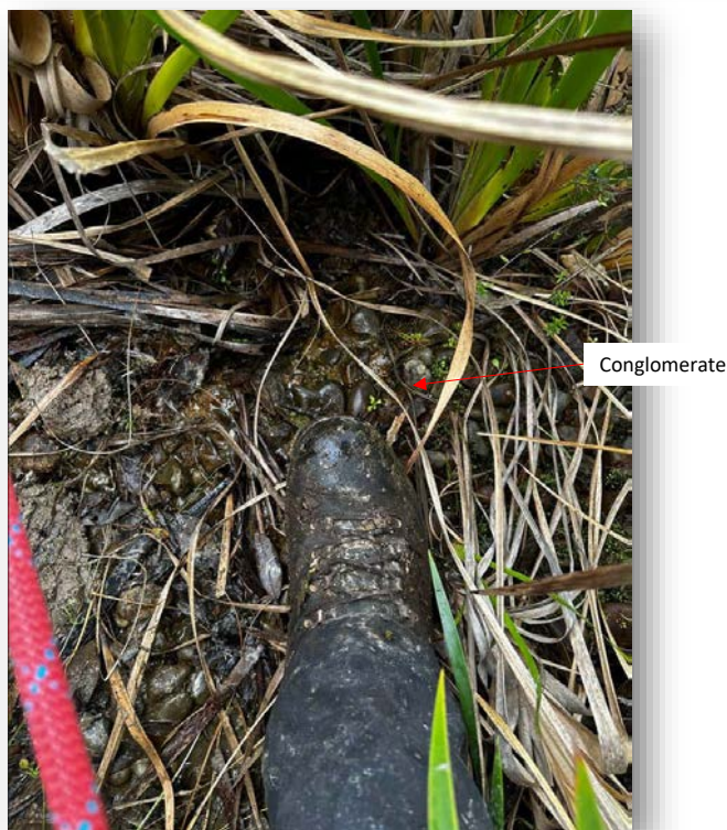
Photo 14: Conglomerate above most recent slip scarp.
