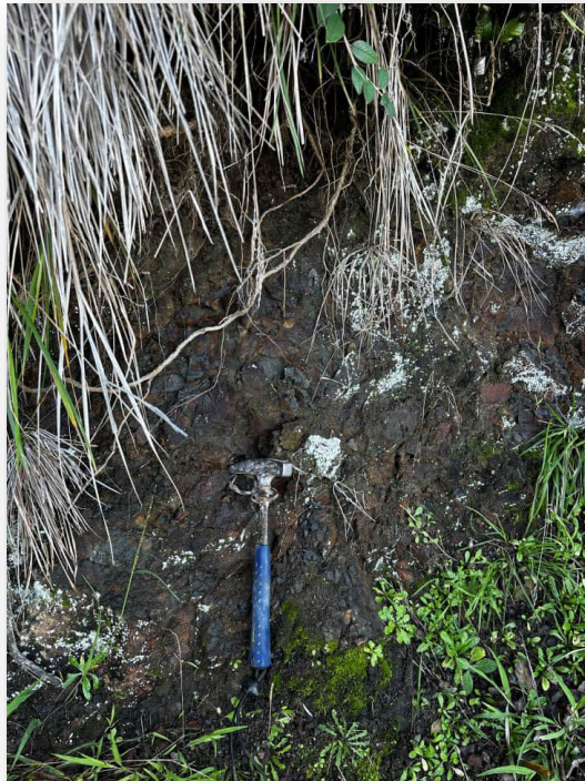
Photo 16: exposed bedrock on the upslope side of the original track alignment across the slip. The rock here is moderately strong to weak, oxidized and generally easy to pick at with a hammer when compared to the outcrop on the foreshore.
