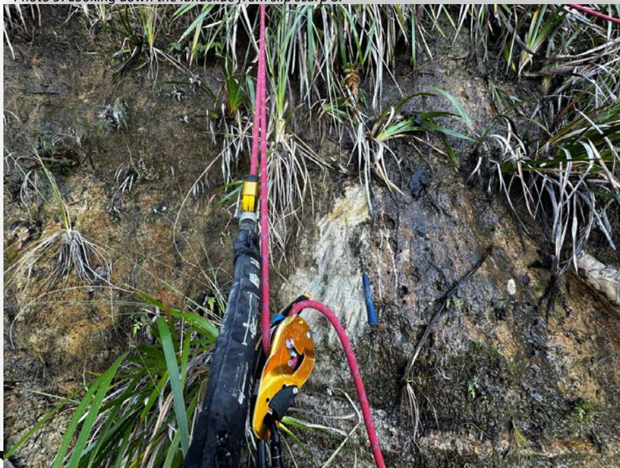
Photo 10: Looking at slip scarp 3. Ground water seepage. Geology hammer for scale and scratching exposing fine sand.
