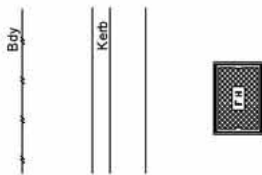
Hydrant in Carriageway
